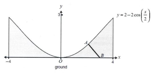
The curve has the equation  $y = 2 - 2\cos\left(\frac{x}{2}\right)$ ,  $-4 \le x \le 4$ . All measurements are in metres; the horizontal length of the structure is 8 metres.
