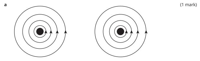
There is a force of attraction between the wires, as the fields are in opposite directions b between the wires. (1 mark)
